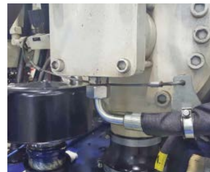
Fig. 2: Caution! Mistake! Incorrectly fitted restraining cable.
