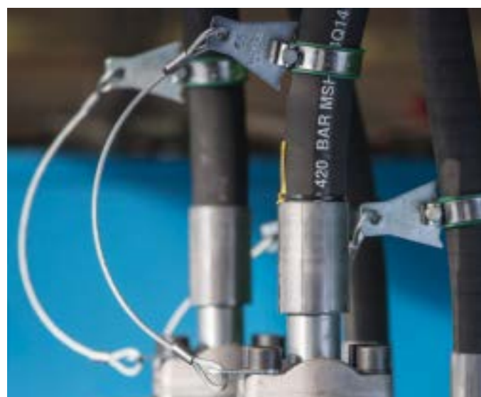
Fig. 1: Correctly fitted restraining cable.
