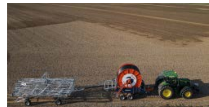
▲ The irrigation systems from Beinlich Agrarpumpen GmbH are mobile. Even the largest combination of drum machine and folded sprinkler wagon permitted for road transport is less than three metres wide.
