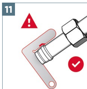
11 Check cutting ring for correct seating using the cutting ring gauge (SRD LEHRE).
